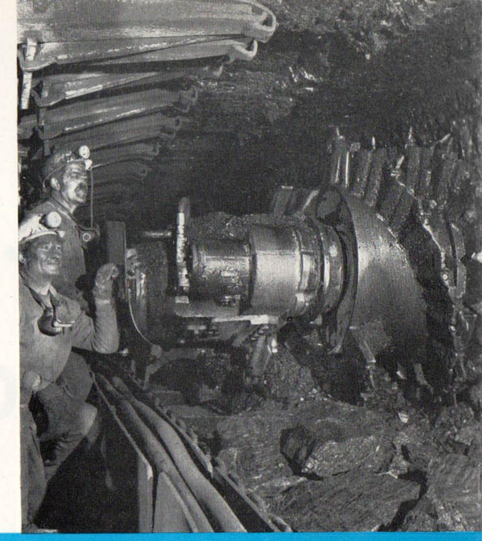
One hundred years in mining vividly portrayed in two photographs . . . (left) the pick 'n' shovel days of hand hewing, (right) a modern production face at Bold Colliery, producing more coal in a day than the miner with the pick could produce in a year.
